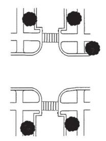
installed either at intersections or mid-block. Curb extensions narrow the roadway to make pedestrian crossing faster and safer. They can be
